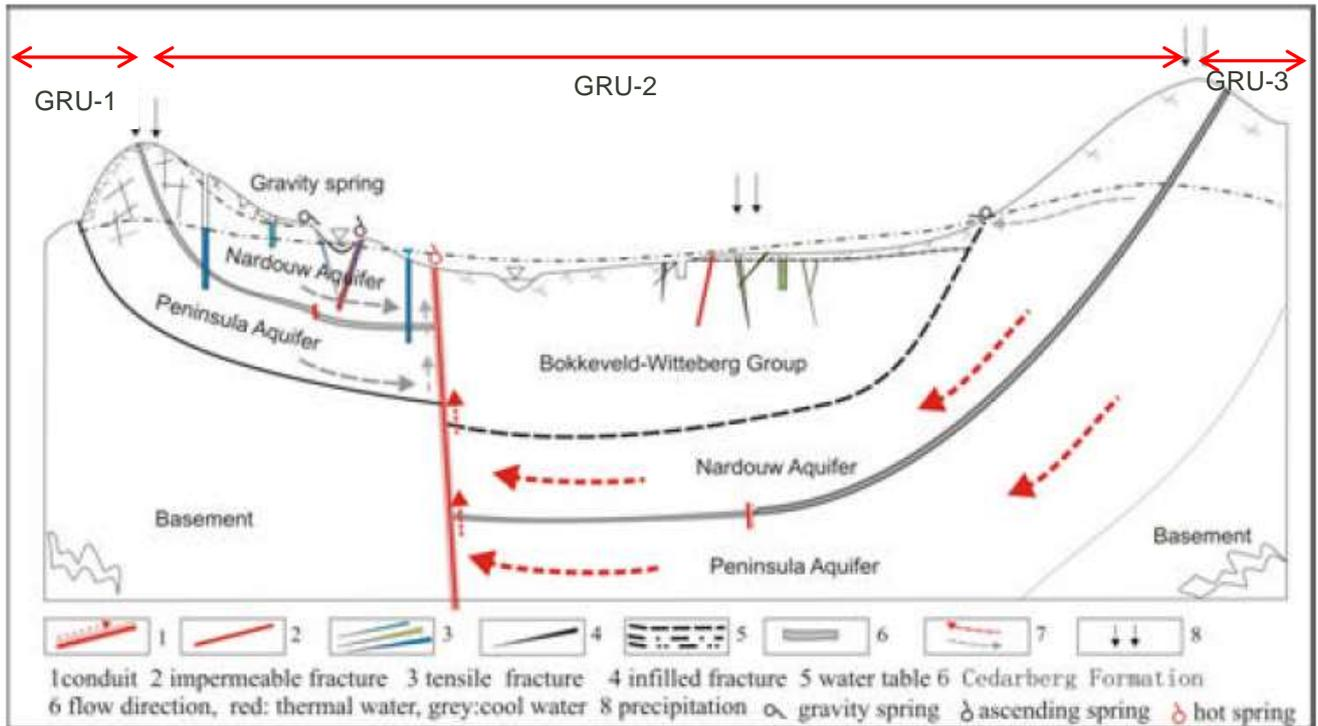
Figure 2-10. Cross-section of TMG flow (Adapted from Wu, 2005).
