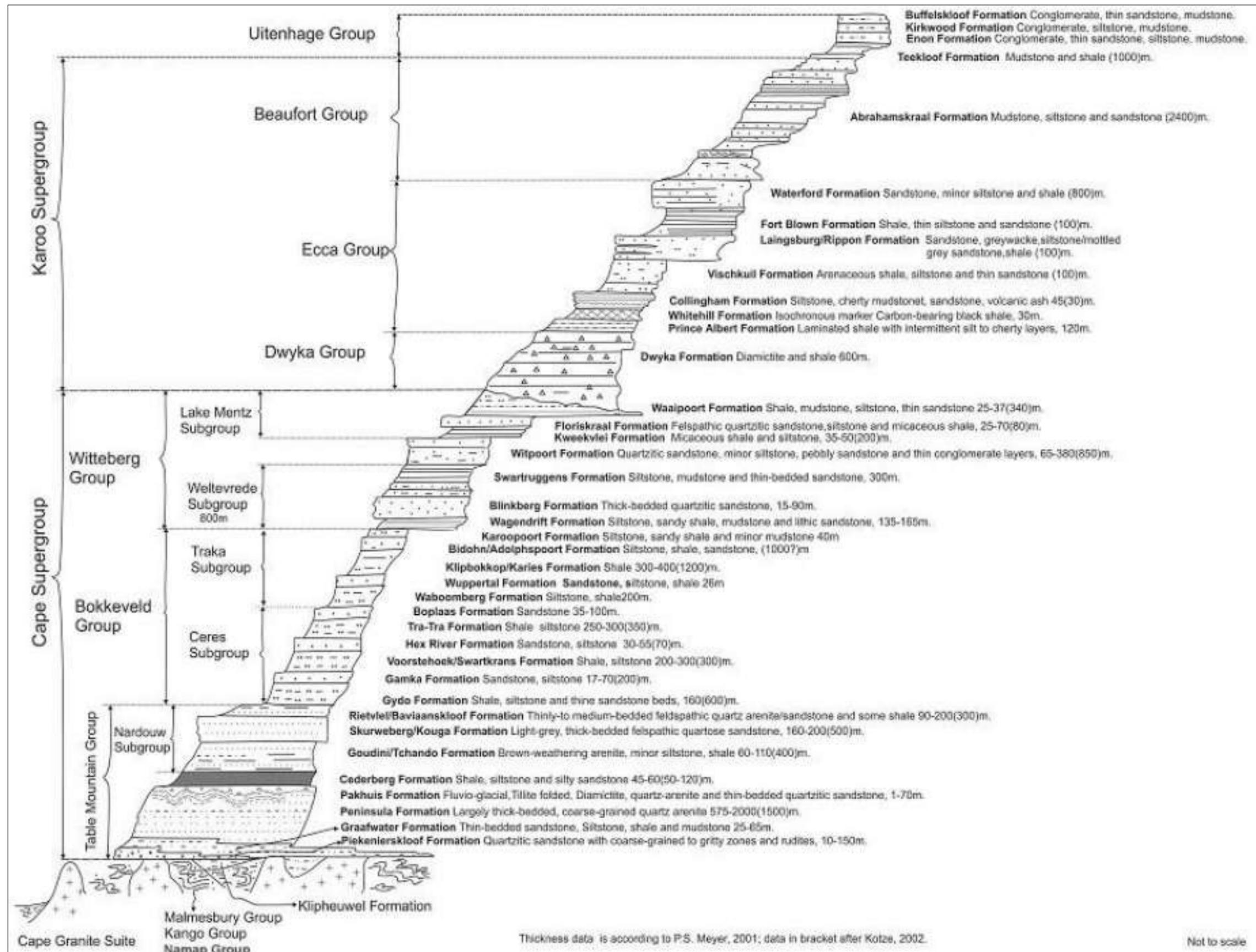
Figure 2-8. Geological sequences in the study area (adapted from Wu, 2005)
